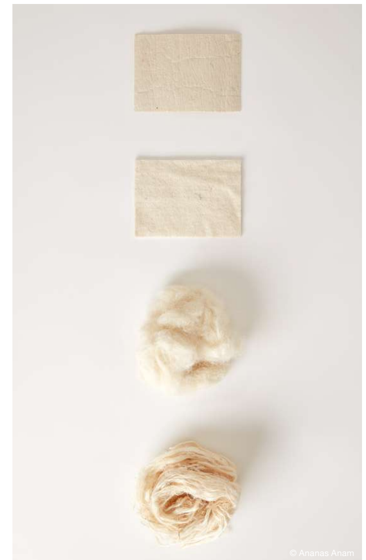
The stages of creating Pinatex, a leather alternative made from pineapple leaf fibres.
