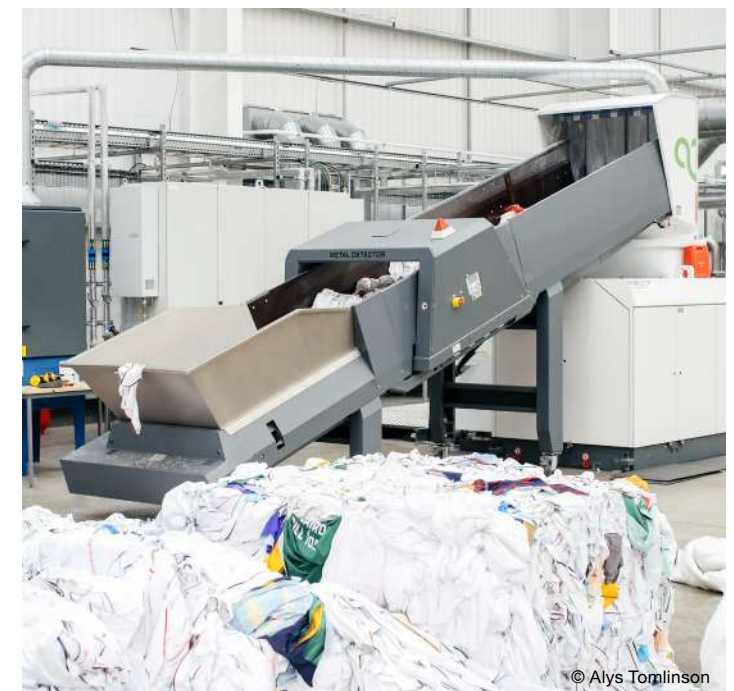
Polyester feedstock, including offcuts from products such as football shirts, ready for shredding and processing into recycled R-PET pellets.
