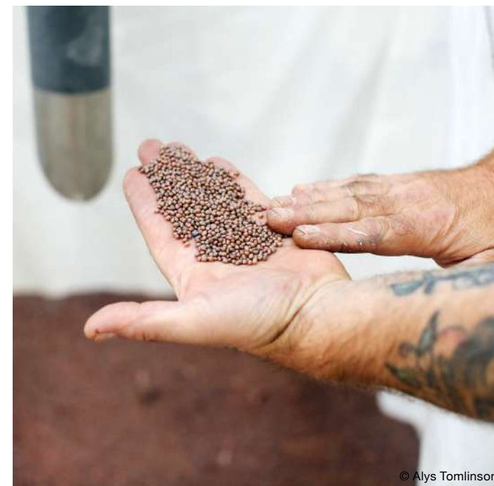
Pelletised R-PET made from post-consumer polyester waste.
